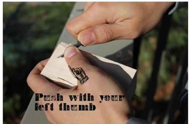
**Stop Cut** – This is a score line that you can cut back to, or make a clear line or feature. Press down and rock your knife back and forth.
