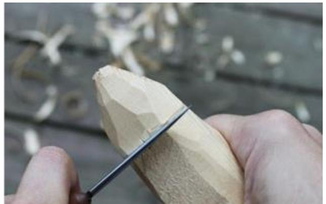
**Shaving Cut** – A cut that ends at a stop cut.
